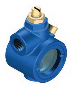
This device is applied for lubrication and cooling systems where oil flow control is necessary. Indication is visual by transparent glasses. The adjusting of the device is very simply by adjusting screw. Clockwise rotation decreases the flow rate, contrary flow rate increases. To avoid turbulence and clogging the adjusted flow should be in one stream and stable. In case of clogging turn off the breather screw until the flow becomes stable.
